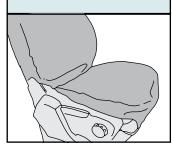
Find the two Velcro straps at the front base of the seat
