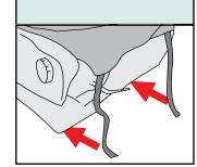
Thread the Velcro strap underneath the seat and fasten to the Velcro at the back of the cover.
