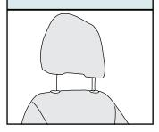
2 Undo side velcro and place cover over seat. Ensure the hole in the side of the seat cover is facing outwards – this must be in line with the seat mounted airbag deployment housing.
