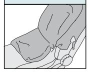
Align cover with plastic headrest insertion points.
