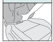
Fasten the side Velcro around the seat adjusters or armrests if applicable.
